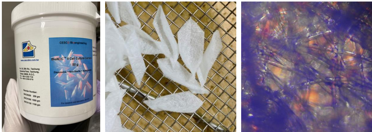
Non-woven PET fabric & Micro-structure (purple: MSC with crystal violet)
