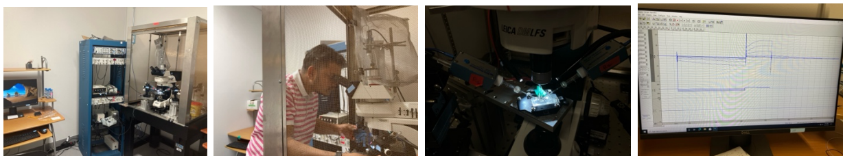
Figure 3: (From the left) The VCF machine full set-up, Data recording is going on, The two electrodes are inserted into the oocyte for data recording, The recorded current from an oocyte.
